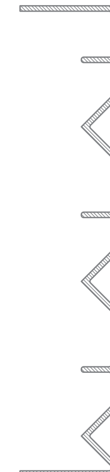
AS10428 Triple Track Sill 0.898 kg/m
