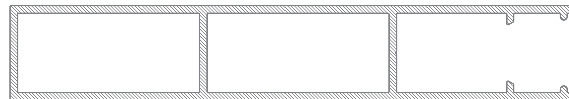
UB025150 25mm x 150mm Batten Outer 2.009 kg/m
