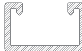
UA10134 41.30mm x 25mm Strut Channel 0.829 kg/m
