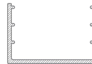
UA2096 38.10mm x 25.40mm Handrail Channel 0.394 kg/m
