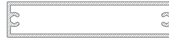
UA6461 75mm x 16mm Railing 0.776 kg/m
