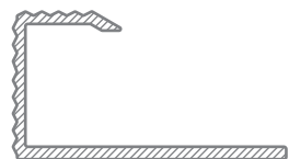
UA4414 13mm Serrated Capping 0.224 kg/m
