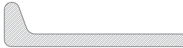
UA2972 76.20mm x 19mm Boat Rigs 1.397 kg/m
